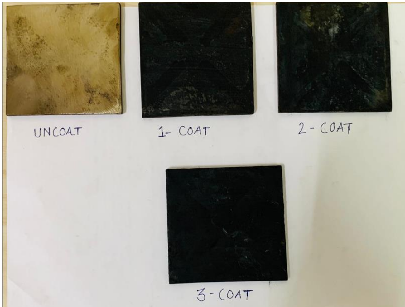
Fig.3b. Actual photograph of Test Plates (After Test)
