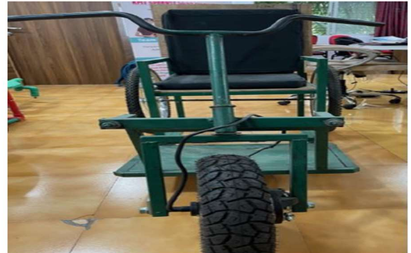
EV cum Wheel Chair for Physical Handicapped Person
